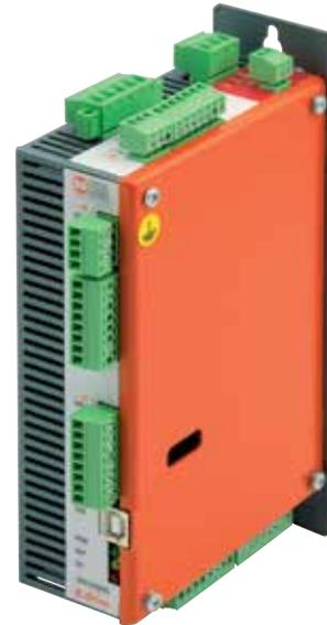
The power stage consists of a mini-step bipolar chopper drive. The e-Drive system features a supply voltage of up to 55VDC for the power supply side and 24VDC for the logic side, compact dimensions and great flexibility of use.
